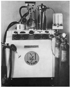
Figure 2.—The Engström respirator as used for anesthesia was equipped with a rotameter block for delivery of oxygen and nitrous oxide to the semi-open breathing system <sup>5</sup> (Permission by publisher).
